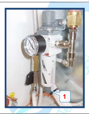
1. Open the valve to water drain
